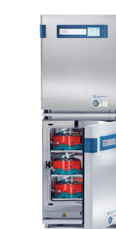
Figure 10. Stacked Heracell Vios CR incubators allow the production of 400 billion cells in about 3 square feet. The results of this testing largely demonstrate the possibility of high throughput parallel processing of cell and gene-modified cell therapies. The modular approach is easily automated and scaled in a highly efficient facility layout. Without intervention, G-Rex bioreactors regularly achieve 40 million cells per square centimeter of gas-permeable cell growth surface area [3]. Each G-Rex 500M-CS can produce 20 billion cells, and each Heracell Vios CR CO 2 incubator can hold 10 G-Rex 500M-CS. Thus, when the incubators are stacked, up to 400 billion cells can be produced in just over 3 square feet of floor space. This predictability enables repeatable, robust, and low-risk cell production for large-scale allogeneic and/or autologous processes.
